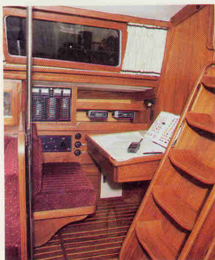
Navigation center has ample space for full electronics. Electric panel is very complete for shore and ship's power.
