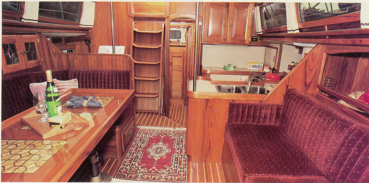
Dining table may be lowered to form an additional double berth. Looking aft, contoured companionway steps are a safety and comfort feature when heeling.
