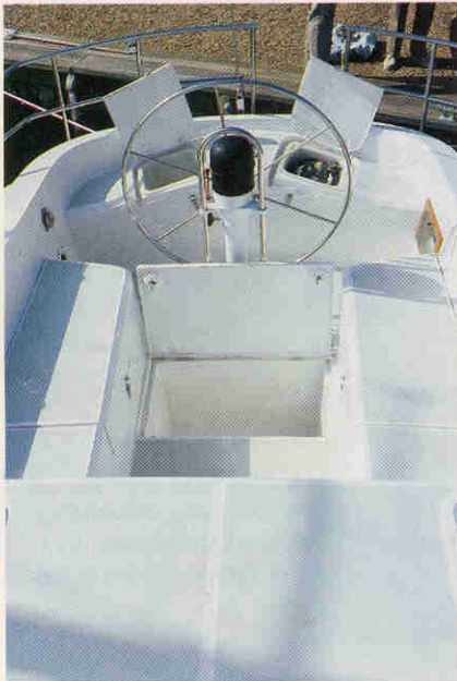
Propane lockers are in the helmsman's seat. Forward of the steering pedestal is a locker for a life raft.
