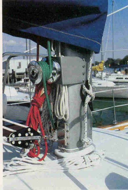
Reefing winch, heavy duty hardware, color coded lines, mast boot make sailing easier and more comfortable.
